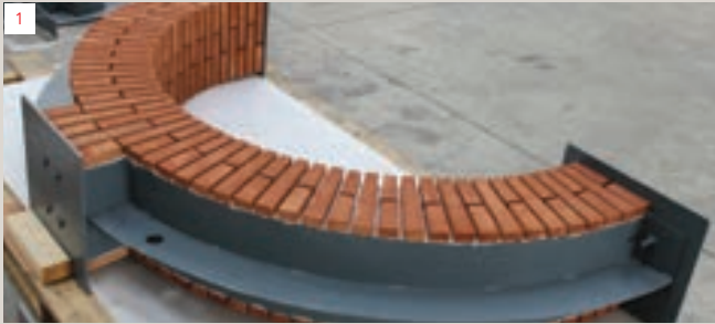
1 Arch with keystone in production 2 Perforated steel lintel 3 Bricks are bonded to steel lintel in factory controlled environment
