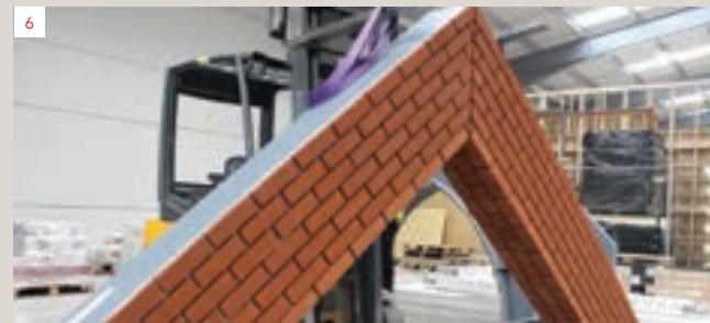
4 Bullseye Brick Slip Feature Lintel 5 IG Brick Slip Feature Lintels in production 6 Brick Slip Apex Lintel
