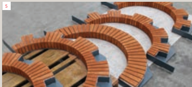
1 Arch with keystone in production 2 Perforated steel lintel 3 Bricks are bonded to steel lintel in factory controlled environment
